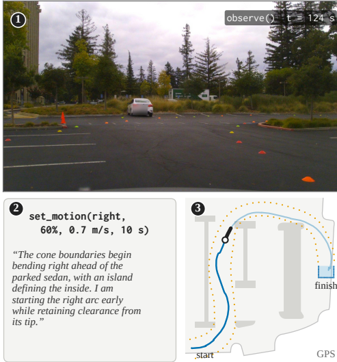
Figure 1: A frontier model driving a car through a fixed cone course. (1) Camera frame returned by observe() . (2) the model calls the MCP to control the car. (3) evaluation trajectory through the fixed cone course.
